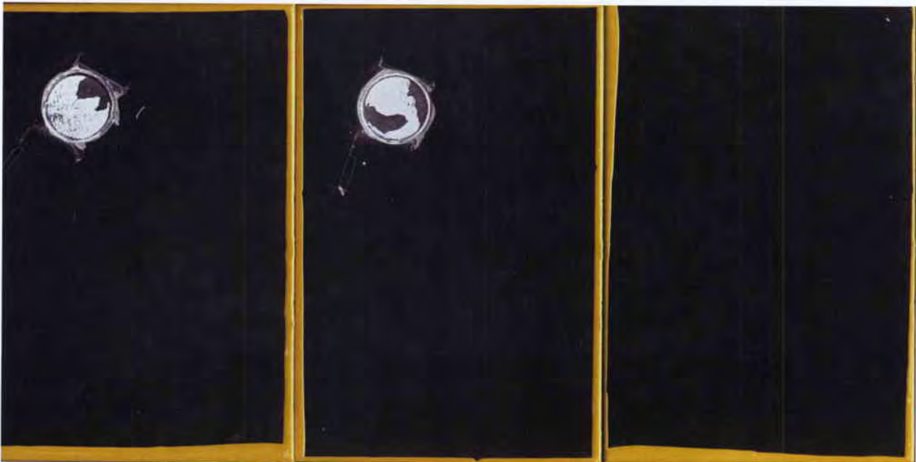
Fig. 3 - Evaluation of samples after water condensation test
